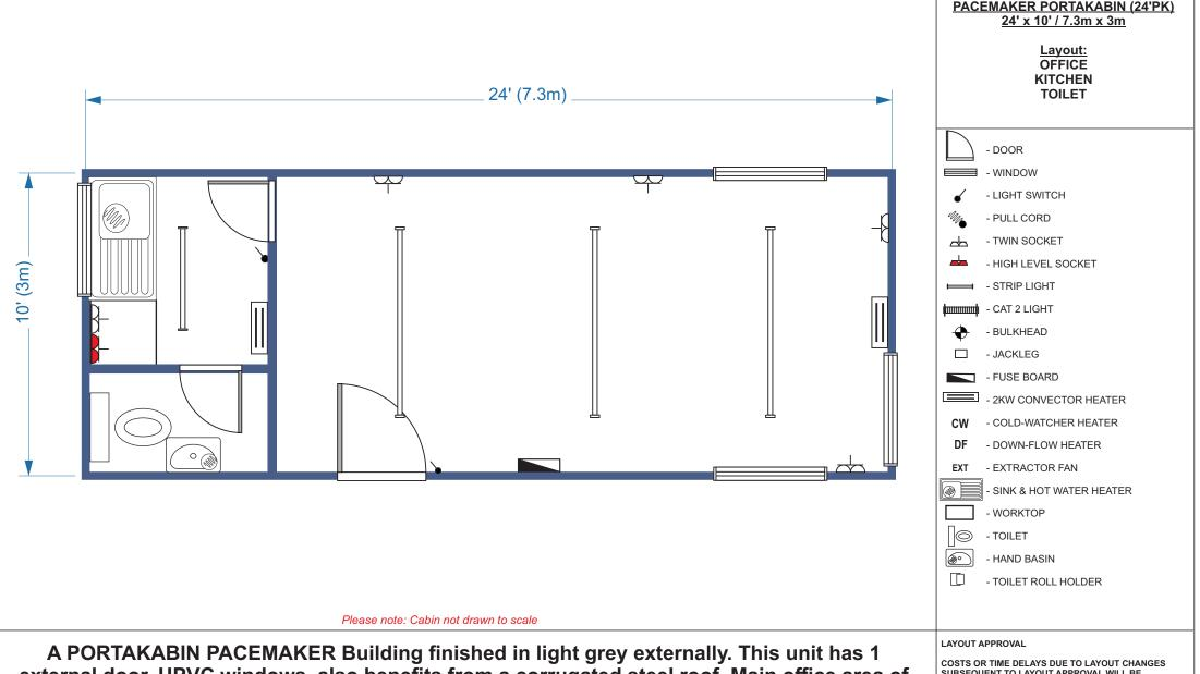
A PORTAKABIN PACEMAKER Building finished in light grey externally. This unit has 1 external door, UPVC windows, also benefits from a corrugated steel roof. Main office area of 16' x 10' giving access to a kitchenette & fully toilet suite, the walls and ceiling are finished in smooth composite steel panels & the floor has a new vinyl covering. Full heat, light & power facilities via a mains fuse board. This unit has recently been fully refurbished & is in excellent condition throughout.
