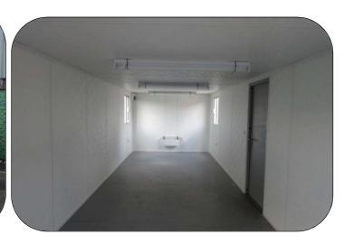
BRAND NEW Steel Secure Open Plan Unit finished externally in grey. Single 'Kirncroft' external steel door with integrated deadlock and keys & 4 sliding windows with double leaf steel shutters. Internally the walls and ceiling are lined with white vinyl faced plasterboard and the floor has grey 2mm polyfloor vinyl, full heat, light & power for mains connection.
